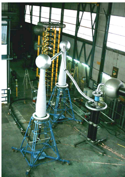
Fig. 4 : Type test of 500 kV premolded joint Partial Discharges Measurement
